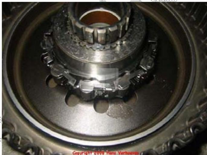
Compress the assembly and install the snap ring for the overrun clutch hub 518.
