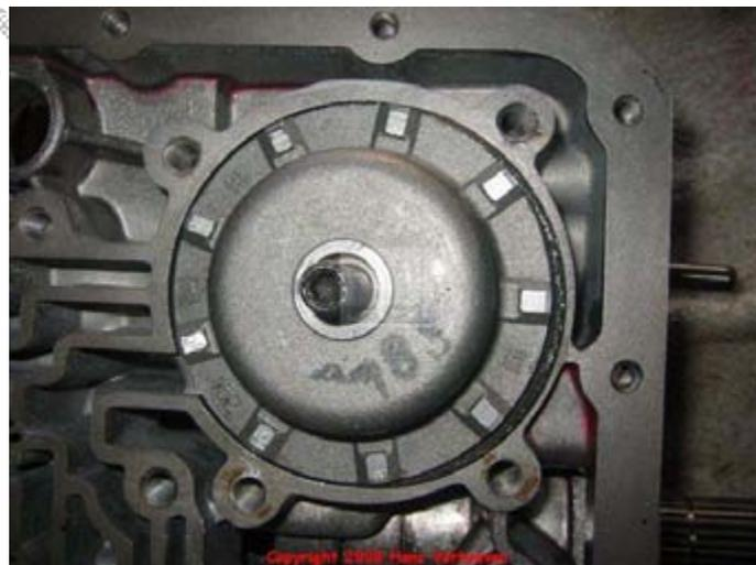
Press on the servo piston 97 to install the retaining ring 93. I used this rather unconventional method of compressing the servo piston 97. Using two of the valve body screws 70 and a hacksaw. You can devise your own way of doing it, but for me it worked rather well.
