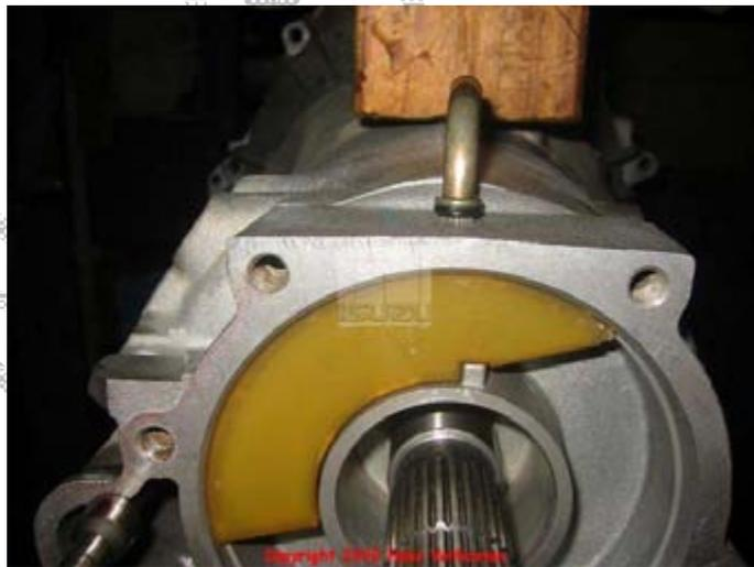
Then install the breather pipe 37 and o-ring 38. The breather pipe 37 holds the reservoir 39 in place, and that's exactly the reason you couldn't get it out in the first place 😊
