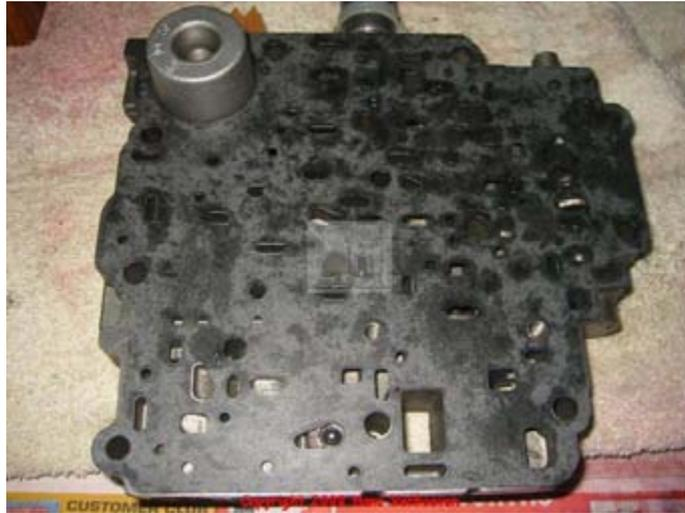
The steel main valve body transfer plate 87 is next. Use the two transfer plate on valve body screws 89 to fasten the plate.
