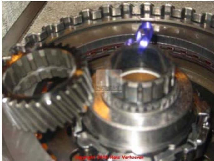
Place the overdrive carrier assembly 525 onto overdrive sun gear 519 i.e. on top of the assembled overrun clutch.
