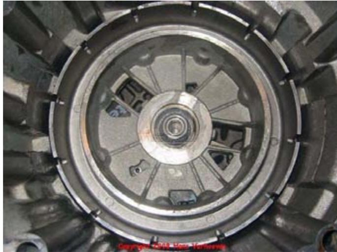
Place the retainer and spring assembly 531 with the retainer facing upwards inside the 4th clutch piston and install the snap ring 530. Ensure it is completely fitted into the groove.
