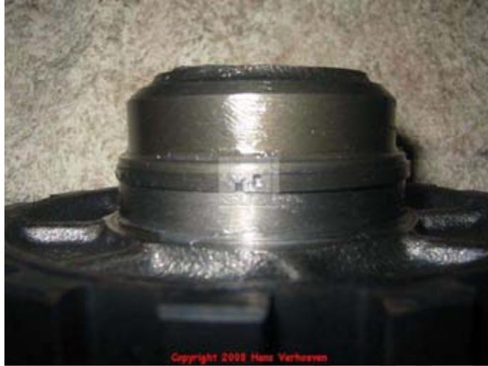
**i** Use a small flat screwdriver to "work" the seal into the case.
