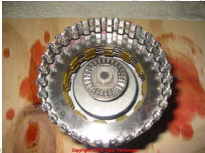
Install retaining washer 636 on bearing 645.
