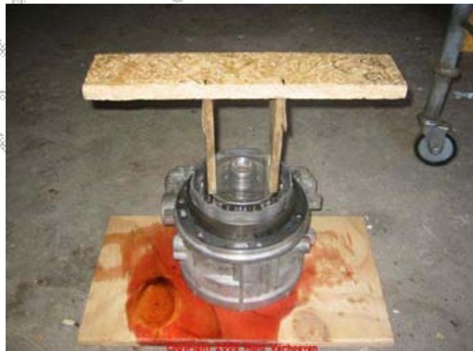
Install the two new oil seal rings 32 on the shaft of the center support assembly. Petroleum Jelly !
