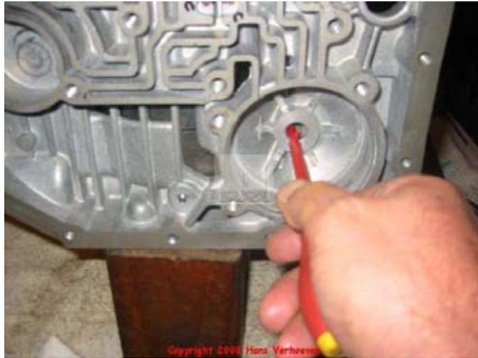
Install output shaft/input sun washer 652 and THEN the output shaft/input sun bearing 651 on top of the planetary carrier using some petroleum jelly.
