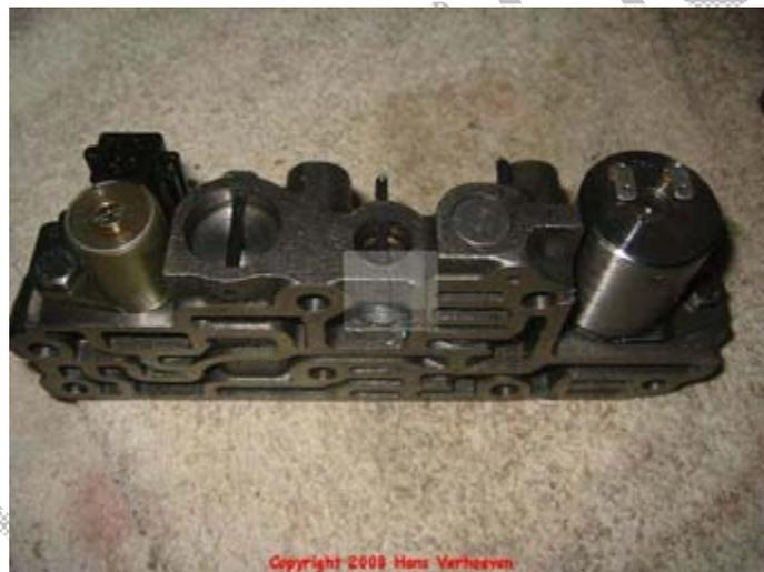
Before sticking the adapter case valve body 401 the wiring harness has to go in place. Route it through the channel in the adapter case before you put the completely assembled adapter case valve body 401 on the adapter case. Stick in the seven screws 70 and hand tighten them.
