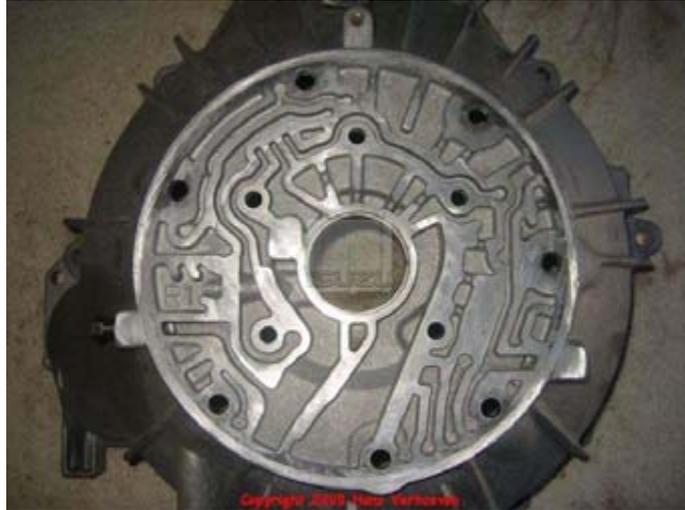
Place the oil pump body wear plate 9. You can not install this one wrong. The holes for the screws won't match up if you tried.
