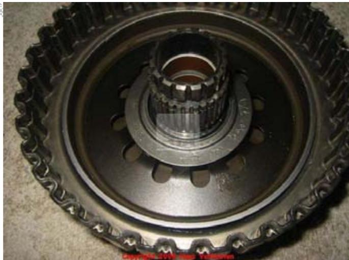
Then the roller assembly 516 goes on top of the release spring retainer 515 in such a way that the overdrive roller clutch cam 517 can be installed after this, check if all of the ten rollers are present !
