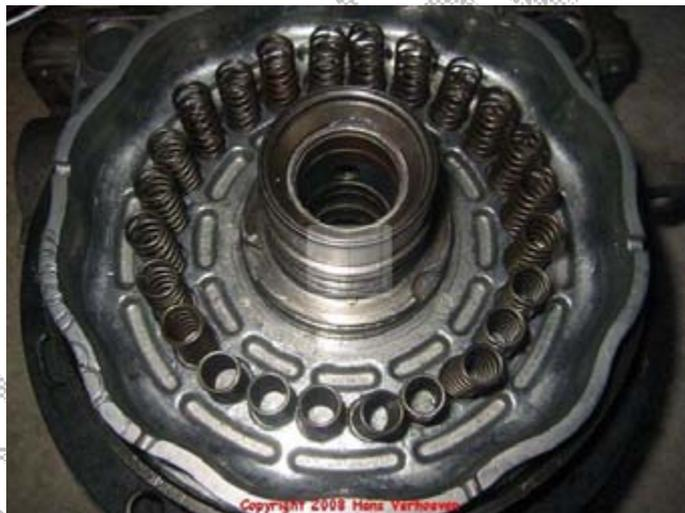
Place all 24 springs 611 into the slots on the inside the reverse piston 610.
