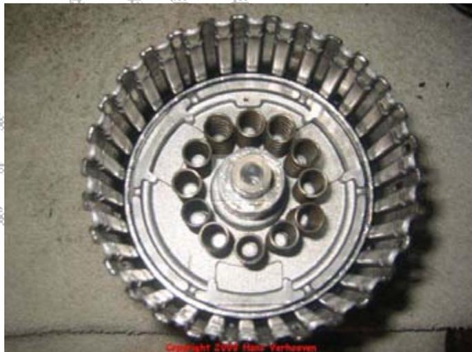
Place 3rd clutch springs seat 639 on the just installed 12 springs.
