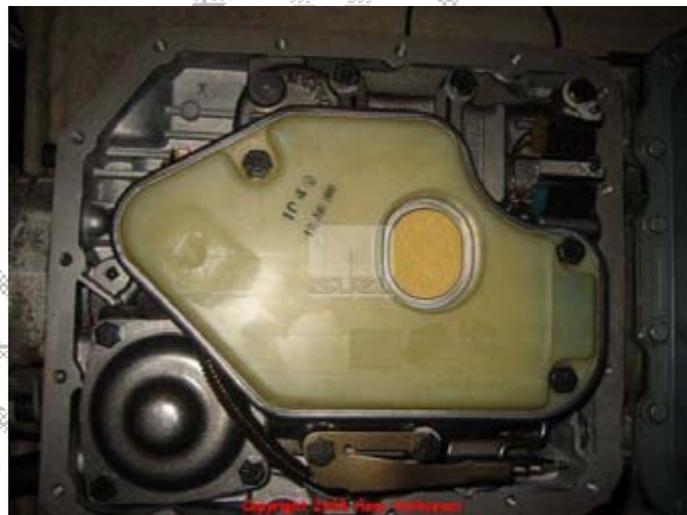
Take the last of the gaskets, the bottom pan main case gasket 75 and the remaining sixteen screw and washer assembly 23. Use 11 Nm. of torque (8 Ft lb or 96 in lb)
