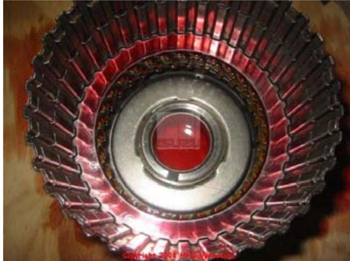
Now place the 2nd clutch spacer 628 on top of the plates.
