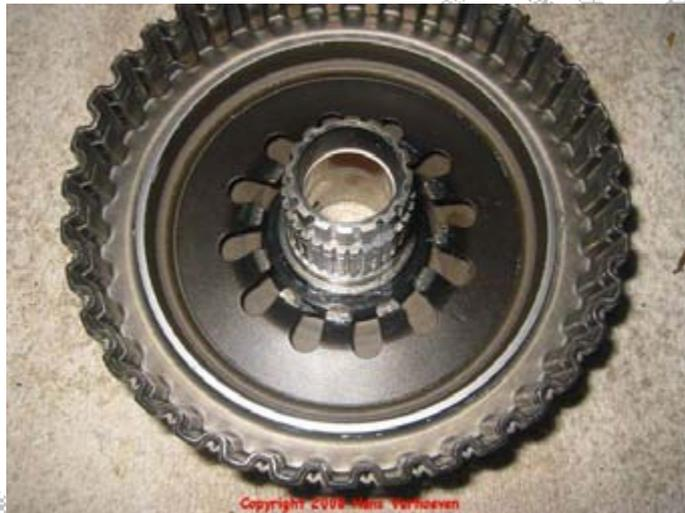
Place release spring retainer 515 with the rim upwards.
