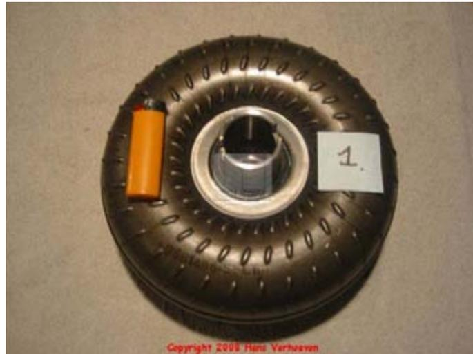
Grease up the splines on the oil pump shaft and slide the torque converter 1 onto the oil pump shaft. Ensure that the converter's shaft is fully seated on the oil pump shaft and give it a couple of turns and very gently take it off again.
