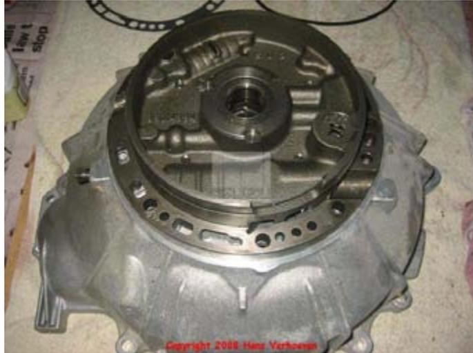
Turn the converter housing 6 on its side and install the five screws holding the oil pump assembly 10. Go hand tight (loose) for now. DO NOT install the converter housing ring seal 3 yet.
