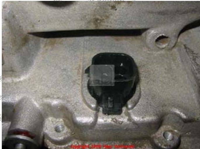
Connect the main case harness assembly 80 to the electrical connector main case 55. Look at the picture for reference on wire colors.
