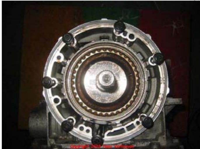
First find out how the steel plates fit in to the adapter case.
