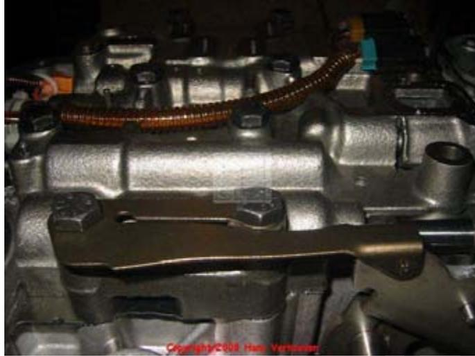
Now you can gently put in 9 of the twelve valve body screws 70 and hand tighten them first. Leave out the three valve body screws 70 that hold the oil filter 79.
