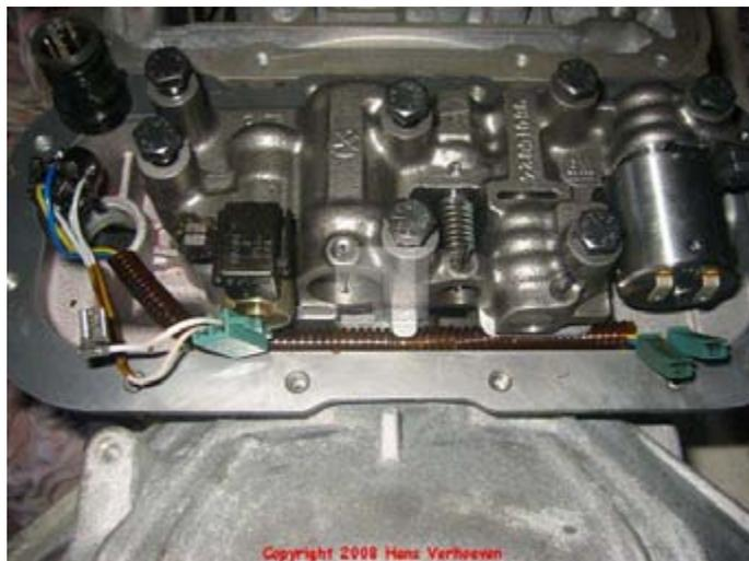
Use a torque wrench set to 20 Nm. (15 Ft lb or 180 in lb) and tighten the seven screws 70.
