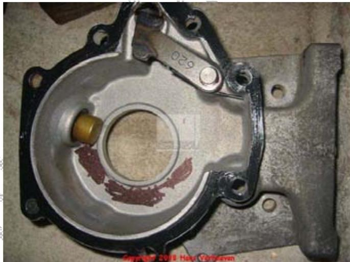
Install the extension case 43 on the main case. Use the seven extension to main case screws 52 and tighten up to 32 Nm. (24 Ft lb or 288 in lb)
