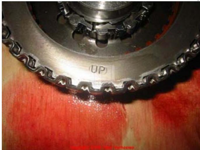
Install snap ring 524 onto the overrun housing.
