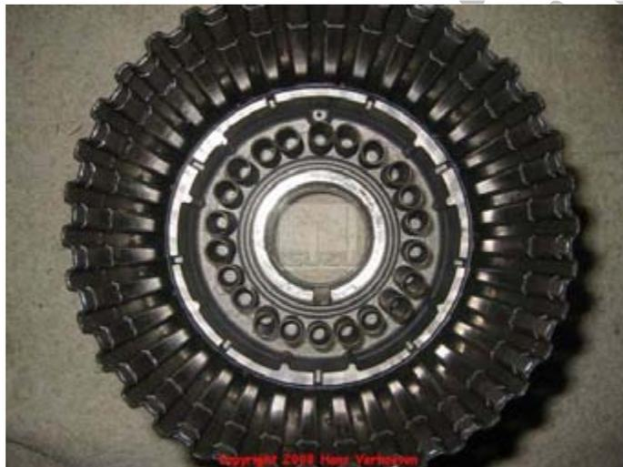
Place 2<sup>nd</sup> clutch spring seat 623 on top of the springs 611.
