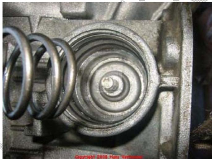
Note: Use petroleum jelly for installation and on the new seals and o-rings.
