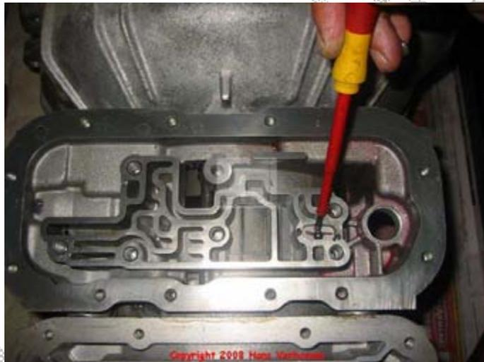
Stick adapter case to transfer plate gasket 104 on the adapter case using petroleum jelly.
