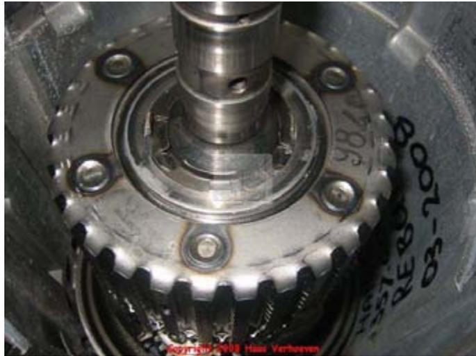
Next put thrust washer 631 on top of thrust washer 632 using the good old petroleum jelly.
