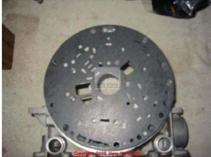
Then stick on the transfer adapter/center support steel plate 29, followed by the second gasket 28. Again use petroleum jelly.
