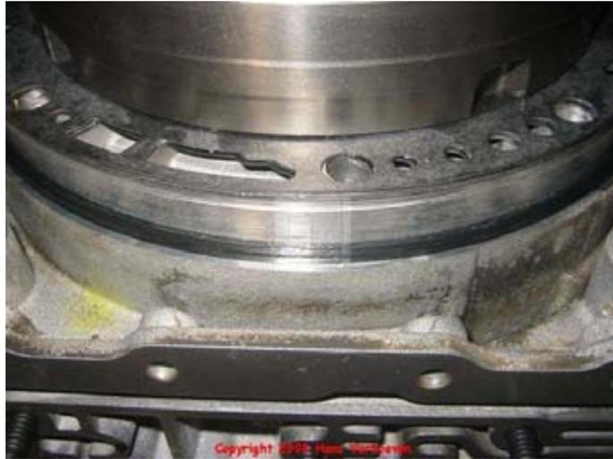
**i** Although the manual shows an actual o-ring/seal 8, the one that came in my rebuild kit was rectangle shaped and proved to work fine. Also look at the drawing of seal locations.
