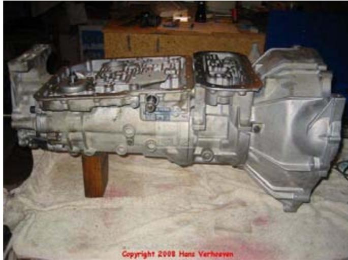
First put check ball 317 in the right spot on the adapter case. See picture for the correct location.
