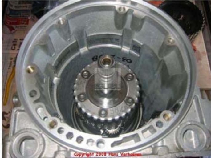
After the 3rd clutch drum assembly is installed turn both the shaft of the 3rd drum assembly as well as the shaft of the planetary carrier a couple of times in both directions. This will ensure proper fit of what is assembled up to now and will also give you a double check on the correct alignment of the teeth in the planetary carrier 653 again. Painting them yellow would have been helpful right now to identify them. Unless you've already done so, get a torchlight.
