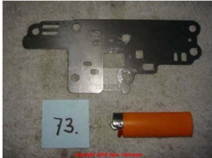
On top of the steel adapter valve body transfer plate 73 goes adapter valve body gasket 72. Again using petroleum jelly.
