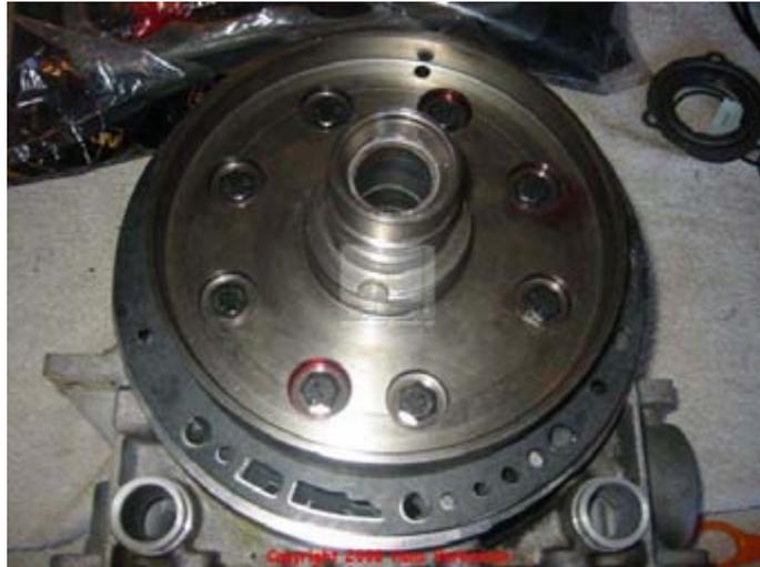
Use the eight screws 31 to fix the center support 30 on the adapter case 20.
