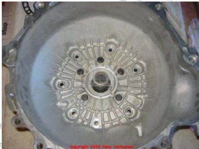
Turn it all back over again and try if you can "wiggle" the converter housing 6 on the oil pump assembly 10 by a few mm. It should have a loose fit for reasons explained later.
