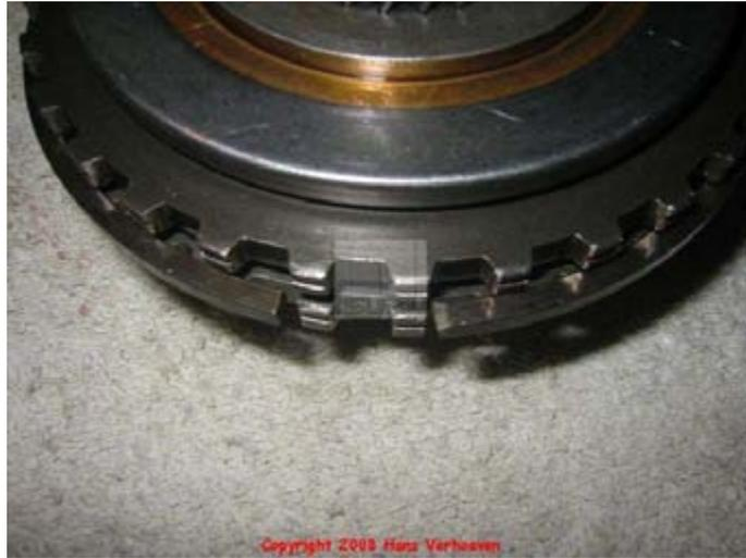
Gently insert, not force, sun gear 646 and sprag race assembly 647 into the 3<sup>rd</sup> clutch drum 634.
