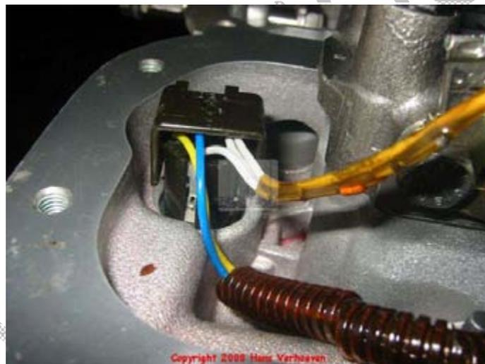
**i** Have you noticed the Fluid temperature sensor in the harness ? It's a temperature sensitive resistor (actually a thermistor)
