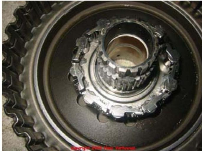
Gently put the overdrive roller clutch cam 517 in the roller assembly 516.
