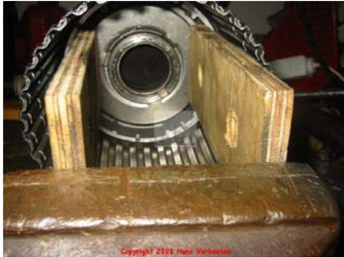
Install the retaining ring 613 and make sure the ring is fully inserted.
