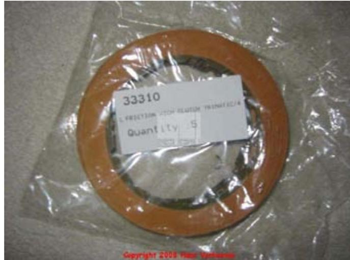
The correct order: steel - lined - steel - lined - steel - lined - steel - lined - steel - lined.
