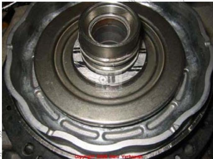
Install o-ring/seal 8 using petroleum jelly !
