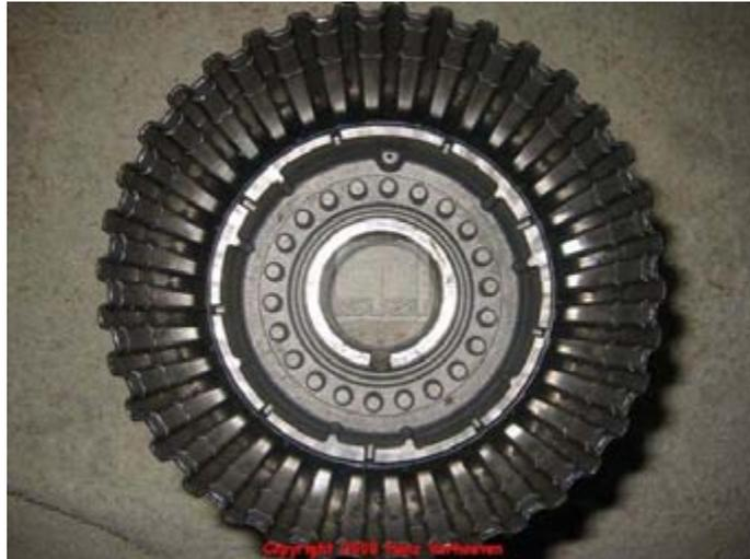
Place the 22 piston springs 611 on the 2<sup>nd</sup> clutch piston 622.
