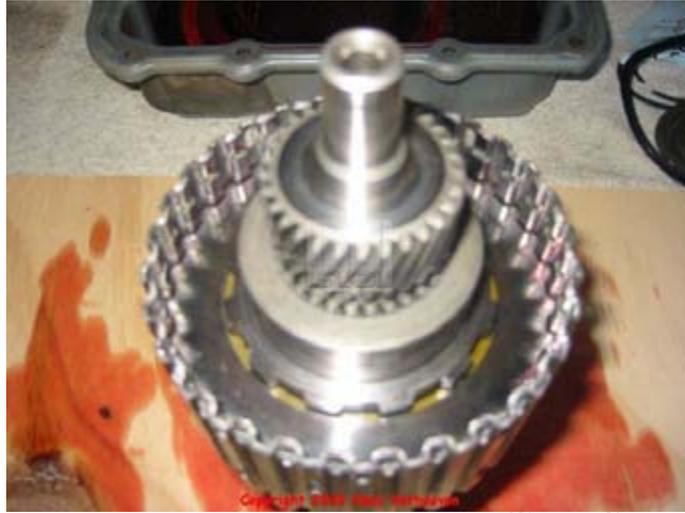
Make sure the grooves of the plates are "in line" with each other. NEVER use force to bring the sun gear all the way down.
