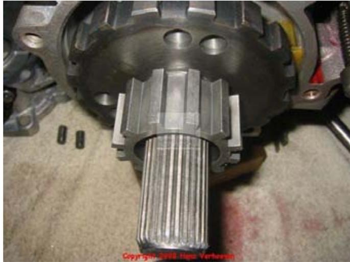
Install the retaining ring 673. On the picture below it's hard to see, but you can just identify one of the little holes in the retaining ring 73.
