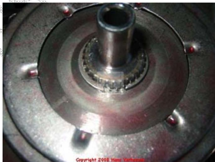
Put thrust bearing 527 on top of the overdrive carrier assembly 525 in a way the turning inner part is touching the carrier 525.
