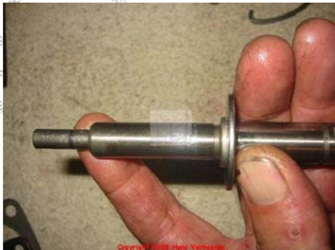
Put the servo piston screw 96 only a few turns into the adjust sleeve 101.
