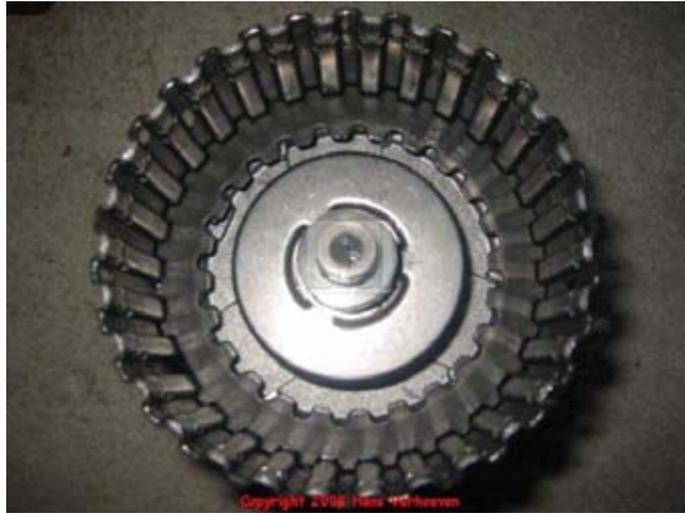
Install retaining ring 640 on inner piston while compressing spring seat 639 down. Make absolutely sure the retaining ring is falling within the cavity of the spring seat.
