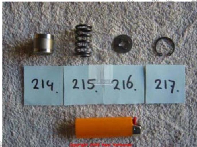
Once you have put all these parts into the oil pump assembly 209 you can install the two oil pump drive gears 201 and 202.
