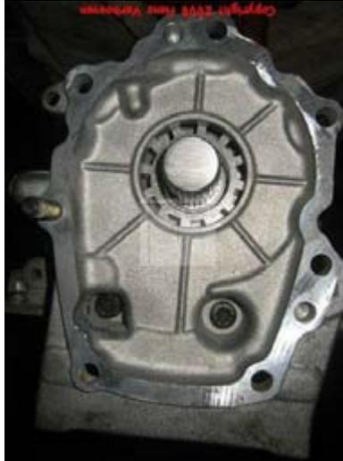
Not covered by the manual are the two steel pint that line up the extension housing with the transfer case. Keep them with the extension case 43.
