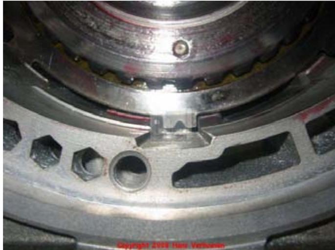
Start putting the reverse clutch plates 615 and reverse lined plates 616 together.
