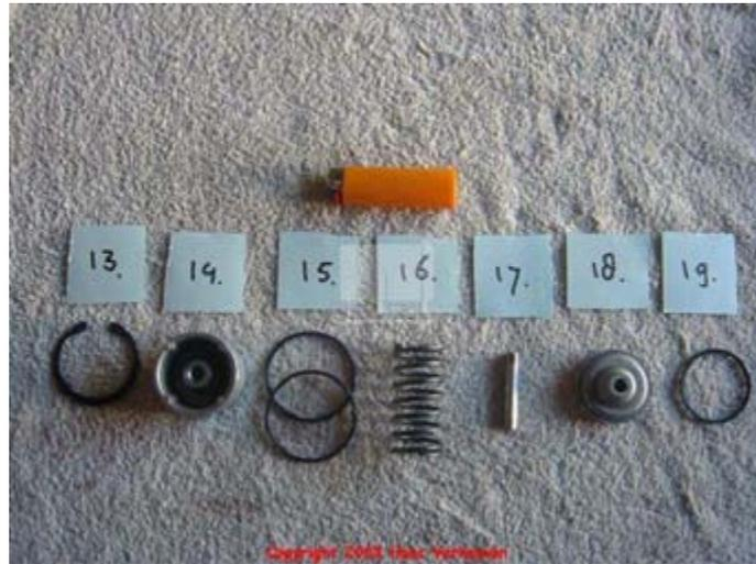
Put the new ring 19 on the accumulator piston 18. Use petroleum jelly. Put the two o-ring seals 15 into the adapter case 20 Using petroleum jelly.
