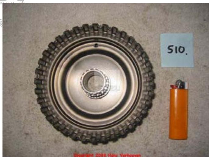
Place the overrun clutch piston 513 into the overrun clutch housing 510 using petroleum jelly.
