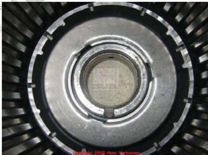
Compress the 22 springs 611. I used a vice and two bits of plywood.
