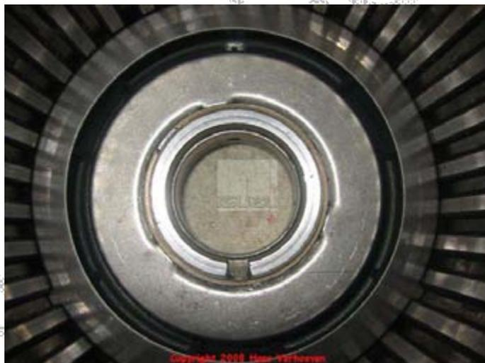
Assemble the 2nd gear clutch pack:
