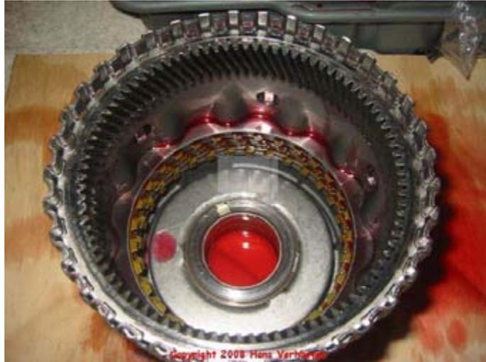
And finally the other retaining ring 629 to hold the ring gear 630 in place.
