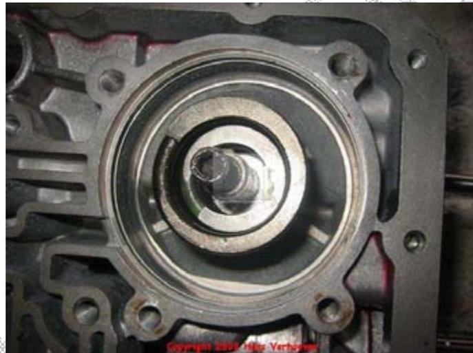
Be careful with the new steel servo piston seal 98. Use a little flat screwdriver to work it into the cylinder.
