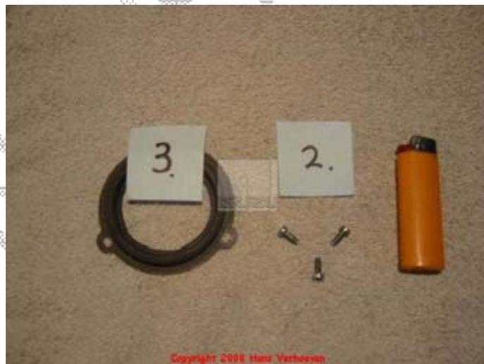
DO NOT try to tap it into place using a hammer or similar. Just use the three screws 2 to EVENLY work it all the way down in it's seat.
