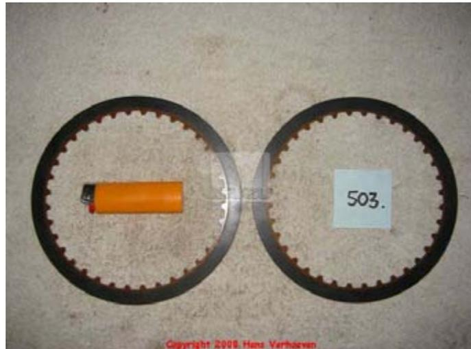
Lower the stack of plates into the adapter case.
