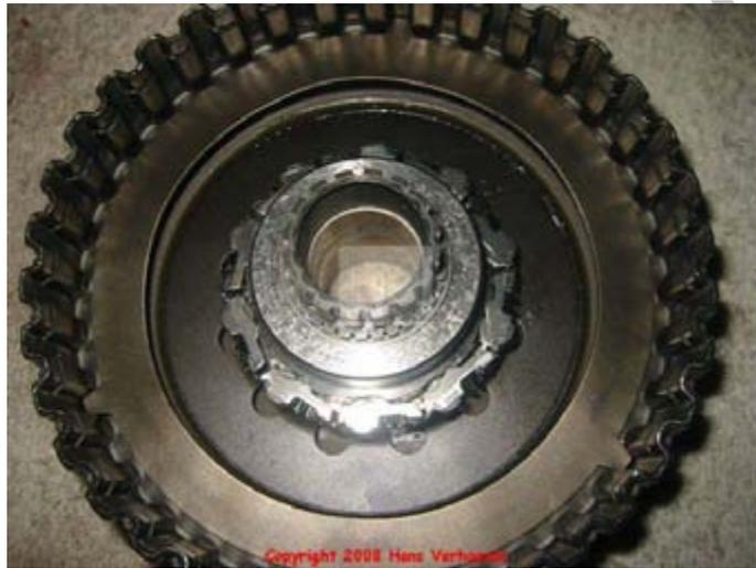
Build up the clutch pack containing steel, lined and backing plate 521, 522 and 523.
