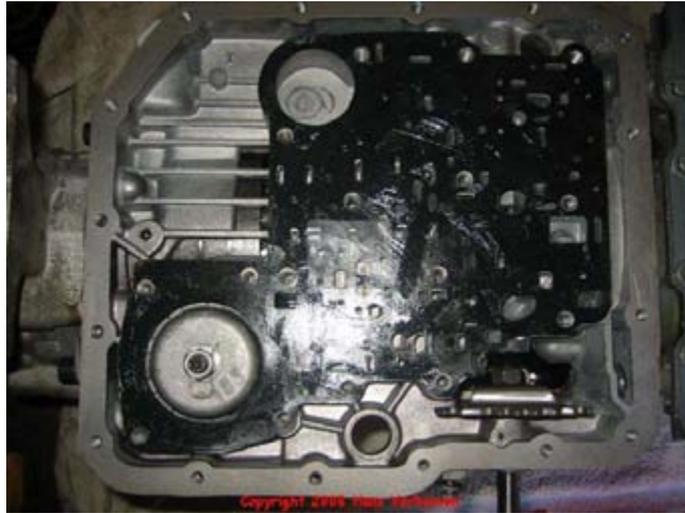
Take the 3rd check ball 317 and place it in the right spot on the main case valve body 301. Again, look at the picture. Use a dab of petroleum jelly to hold it in place and prevent it falling out.
