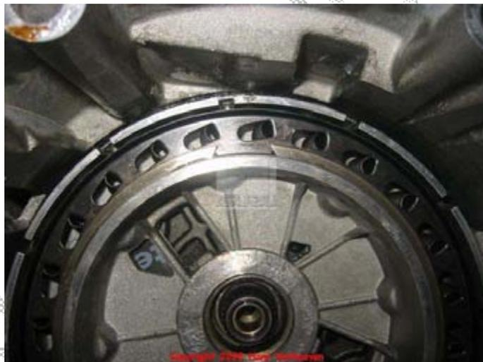
Stick in the thrust washer for the internal gear/support 529. Tangs facing down. Use petroleum jelly to prevent it falling out.
