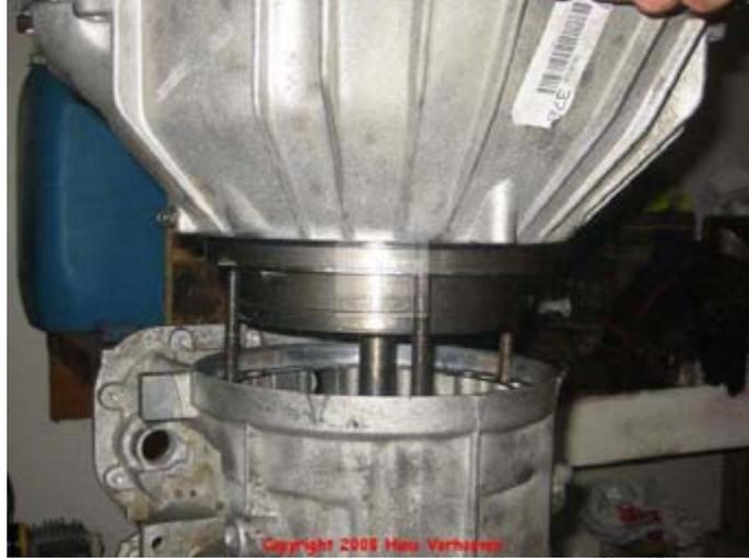
Once the converter housing 6 is installed on the adapter case 20, take the remaining screws 4 and slide them into the converter housing 6. It's a good idea to put petroleum jelly on them.
