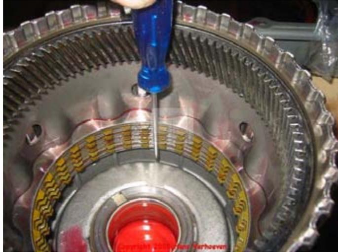
Just slide it in without any kind of force. The grooves of the 3<sup>rd</sup> clutch assembly will easily slide onto the lined plates 627 of the 2<sup>nd</sup> clutch assembly. Carefully slide it in further until the teeth of ring gear 630 slide on to the teeth of the planetary carrier 653.
